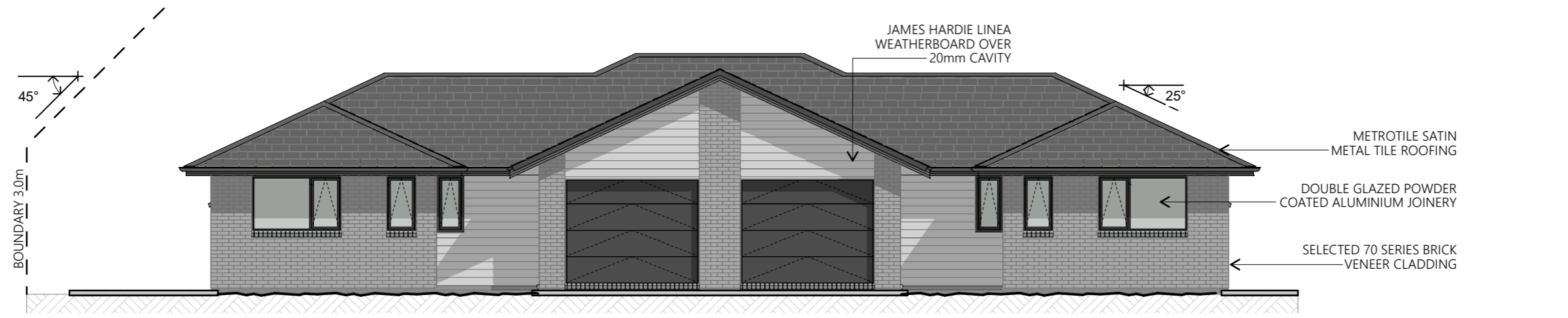
NW NORTH WEST ELEVATION U1-2 / U3-4
